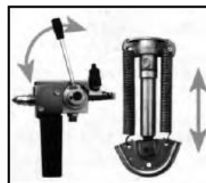
Hydraulic braking system with tractor pedal if supplied 8000-10000-12000-14000 kg PN 020
