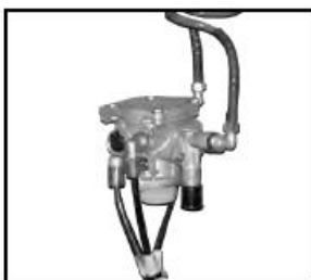
Pneumatic braking system 8000-10000-12000-14000 kg PN 008
